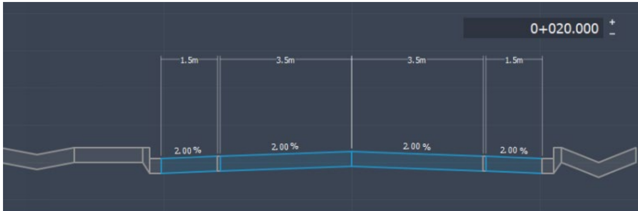
Figure 8 10.0m Wide Road with Curb & Gutter
