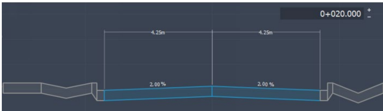
Figure 6 8.5m Wide Road with Curb & Gutter
