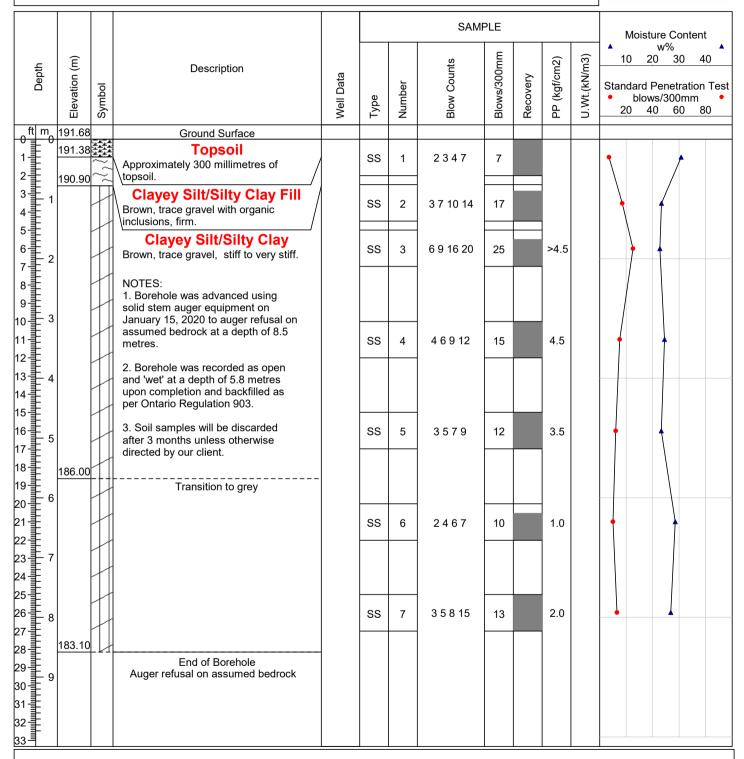
Drill Method: Solid Stem AugersDrill Date: January 15, 2020Hole Size: 150 millimeters
