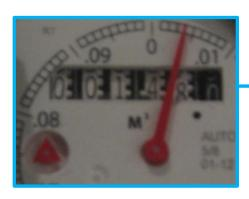
A close-up of the register to the right would indicate a reading of 00148.004 or 148.004 cubic metres.
